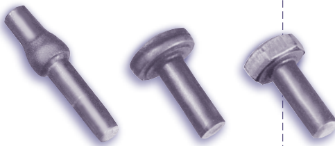
Fig. 55 A single-die, two-blow heading machine forms the wafer section on this hex head cap screw on the first upset. The cold-formed part is then transferred to a trimmer where the hex is formed.
