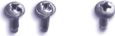
Fig. 49 These Phillips® head sheet metal screws made from Type 305 stainless show the difference between cold and warm heading. The one on the right was warm headed successfully. The two on the left, however, were cold headed and have obvious defects. Stress cracking is the cause, not surface imperfections.
