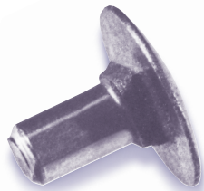
Fig. 51 Warm heading eliminated stress cracking for the severe upset of this truss shoulder bolt made from Carpenter No. 10 stainless.
